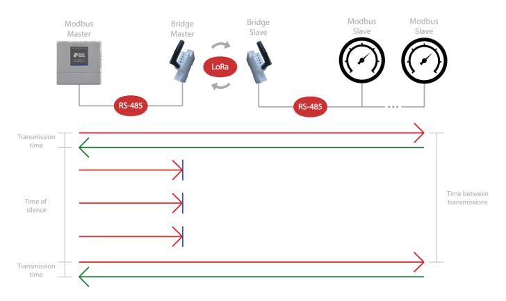
Based on these times, we establish 2 communication rules that must be applied at the Modbus Master. The first one is completely mandatory in order to establish communication with the Modbus slaves through a Bridge LR network:
